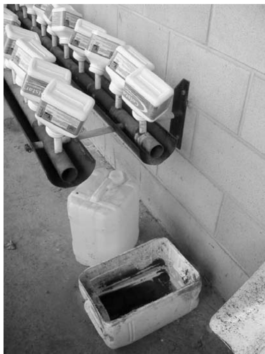
Figure 9: This simple, DIY-built system allows plastic chemical containers to be triple-rinsed and drained with the run-off collected in separate vessels.
